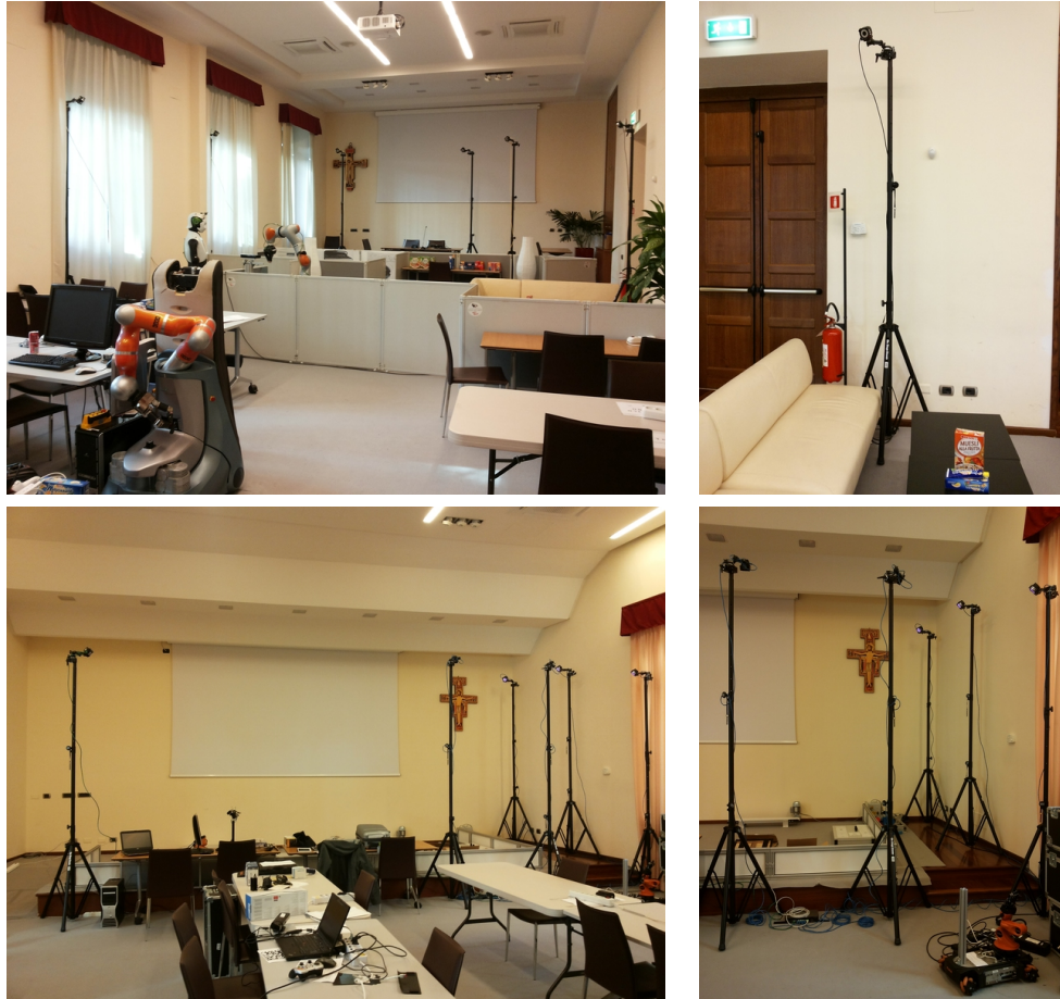
Figure 2.3: Motion capture cameras as installed at the 2014 RoCKIn Camp. On the left, camera setup around the RoCKIn@Home (up) and RoCKIn@Work (down) testbed. On the right, closer views of a single RoCKIn@Home tripod with camera (up) and of part of the RoCKIn@Work setup (down).
