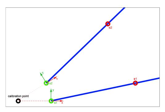
Figure 2.16: Example of two different starting points, s1 and s2. Note that the orientation of the path depends on the starting point.
