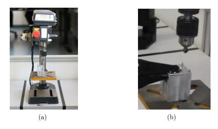
Figure 2.4: The RoCKIn@Work drilling machine (a) and a cover plate which is placed in the fixture of the drilling machine (b).
