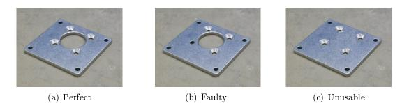
Figure 2.6: Three possible states of the cover plate
