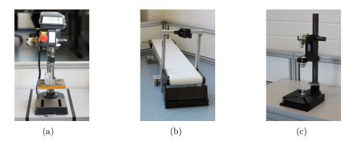
Figure 1.2: Networked devices at the RoCKIn@Work environment. (a) Drilling machine (b) Conveyor belt and quality control camera (c) Force fitting machine
