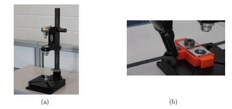
Figure 2.3: The RoCKIn@Work force fitting machine (a) and bearing boxes in the middle of force fitting process (b). The first bearing (right side) has been successfully force fitted into a bearing box.
