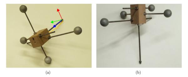
Figure 2.13: The marker set used in FBM3. The rod is marked by the yellow brace. The tip of the marker set is marked by the origin of the coordinate frame (the orientation of the coordinate frame is irrelevant here).
