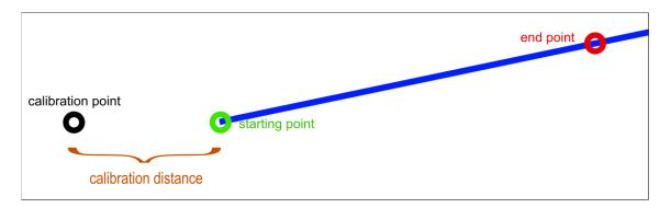
Figure 2.14: Example of a path on a straight line.
