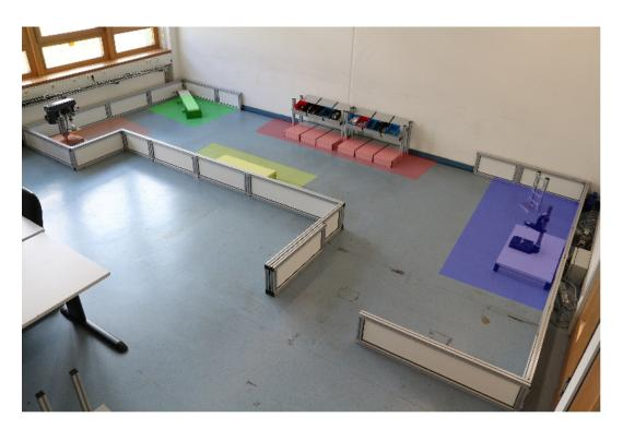
Figure 2.2: Example of the spatial areas in RoCKIn@Work environment. The spatial areas are shelves (red), force fitting workstation (blue), conveyor belt (green), drilling workstation (orange) and assembly workstation (yellow).
