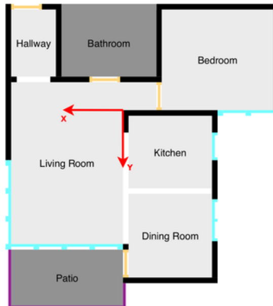
Figure 7: Example of a testbed reference frame for RoCKIn@Home. The z -axis points towards the reader.
